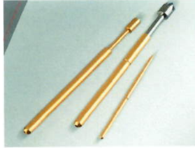
STANDARD TEST PROBES 30 MIL - 177 MIL (0.76 MM - 4.50 MM)
